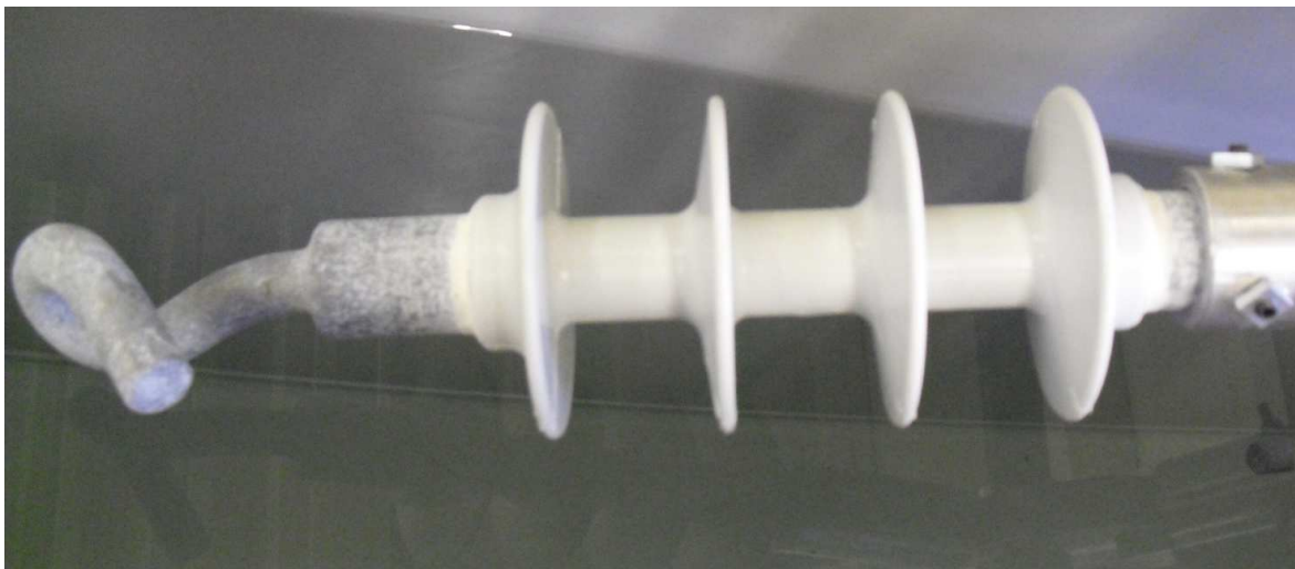
Figure 5.1: Flat insulator (insulator n°1 in the test)
