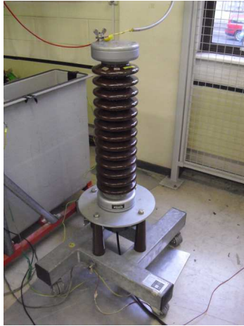
Figure 4.4: Snapshot of Voltage Divider (ratio 3750:1)
