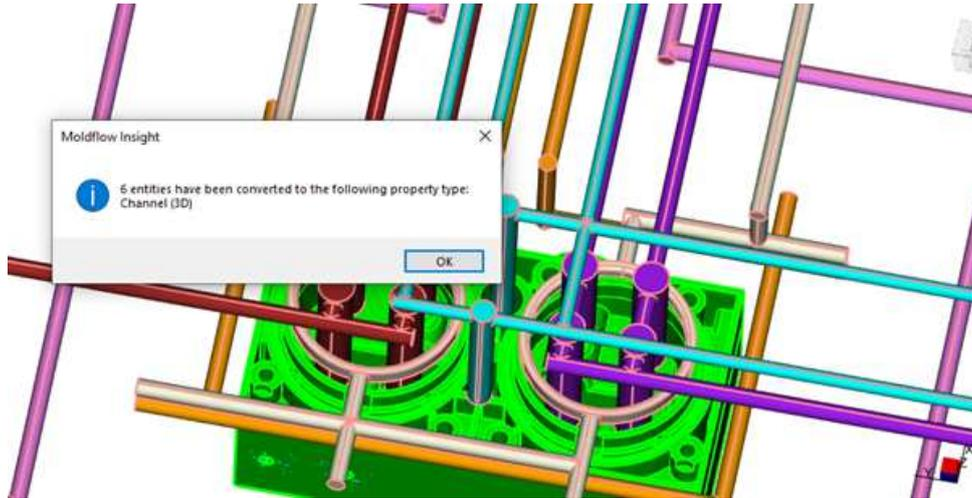
Figure 4.5: Change property for the imported channels before the mesh. This passage can be achieved by >select the complete geometry of one channel >right click on the selected area >change properties >channel or 3D channel.
