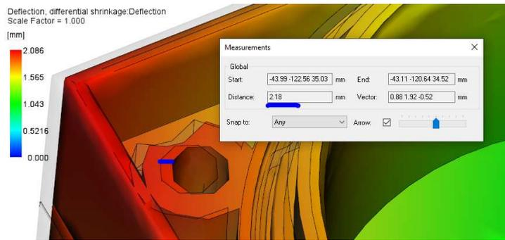
Figure A.6: Detail of the deflection for differential shrinkage.
