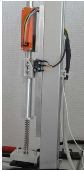
Figure 4.3: Tele-echography robot, linear actuator used for the end-effector.
