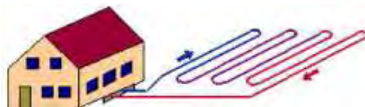
Figure 21: Horizontal layout of a BHE (Sanner, 2001)
