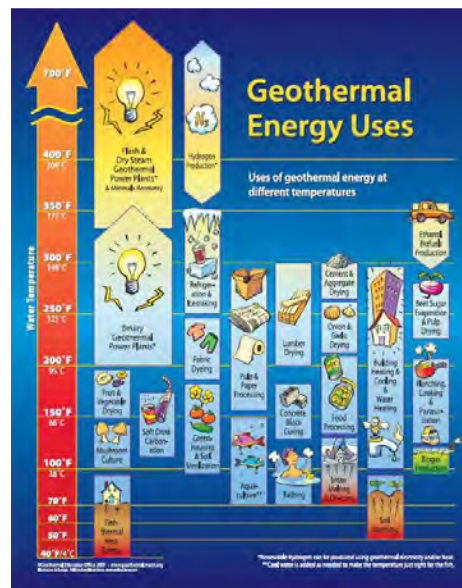
Figure 18: Various geothermal uses, including power generation and direct use, related to their appropriate temperature range (Lund, 2011)
