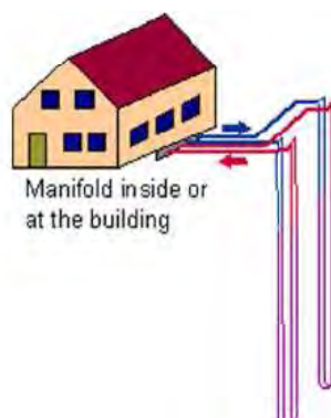
Figure 22: Vertical layout of a BHE with double U-pipe concept (Sanner, 2001)
