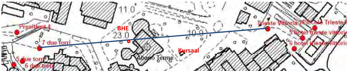
Figure 38: Section between the two wells considered to estimate the stratigraphy beneath the Kursaal
