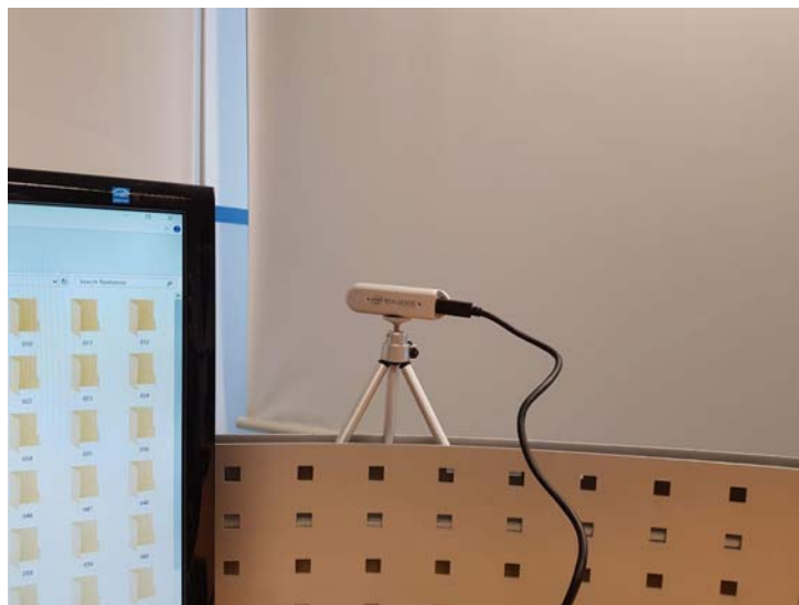
Fig. 6–1: D435 set up to perform the White wall test, where the camera was put in front of a flat projection screen to analyze the quality of the resulting depth map while detecting a known surface
