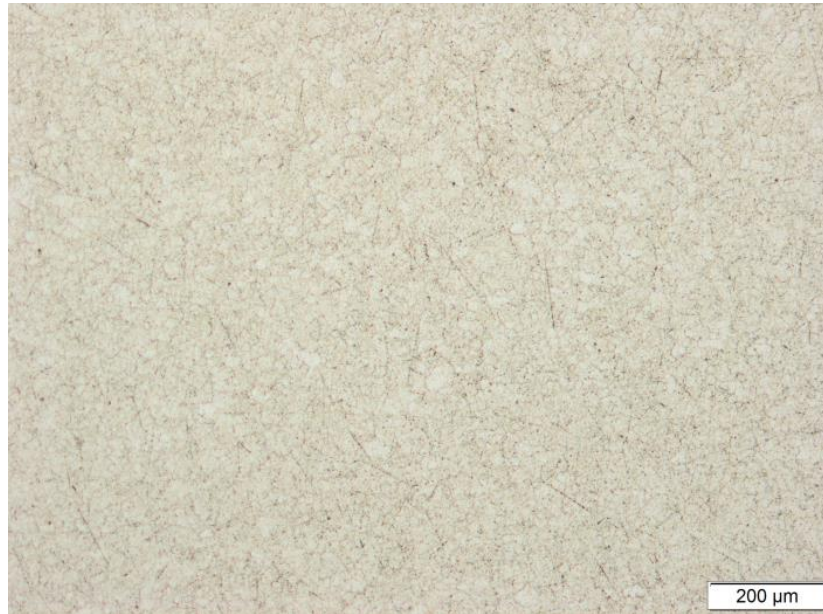
Figure 4-7 Sample 11-5 etched in 0.5% HF (conc.) in water for 3.5min, 5X. The grain boundaries are not sufficiently highlighted for a good estimation of the grain size.
