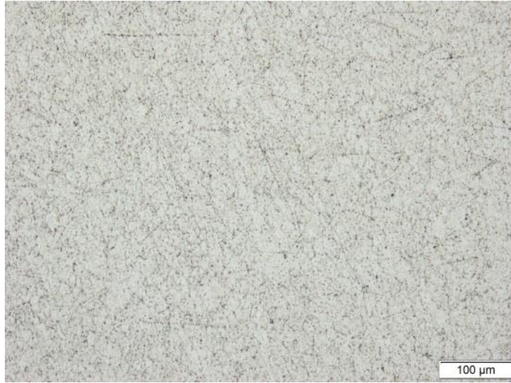
Figure 3-6 Effect of the etching with the Keller's reagent. The sample were uniformly corroded without highlighting the grain boundaries.
