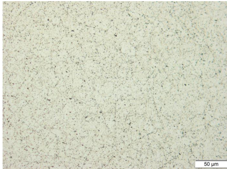
Figure 4-9 Sample 11-5 etched for 2.5 min, 20X. Here is more clear that the corrosion of the samples is not localized on the grain boundaries but tend to be more uniform all over the surface.
