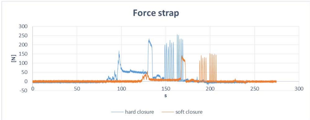
Figure 3. 14 Difference of force on Velcro strap
