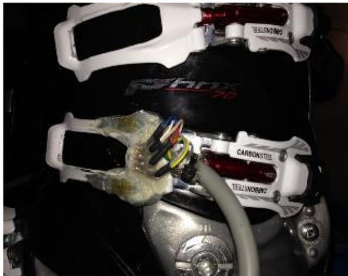
*Figure2. 6 Strain Gauges applied on the buckle of the boot*
