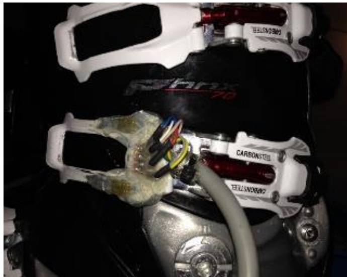
Figure2. 6 Strain Gauges applied on the buckle of the boot
