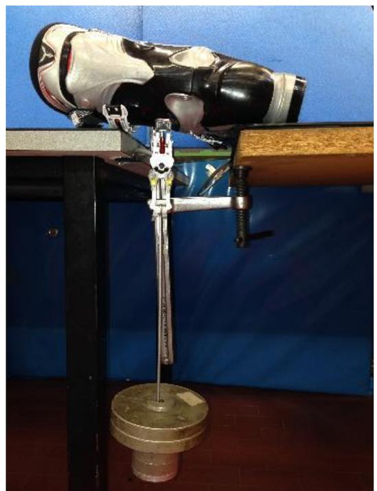
*Figure2. 8 Masses application for the buckle calibration*
