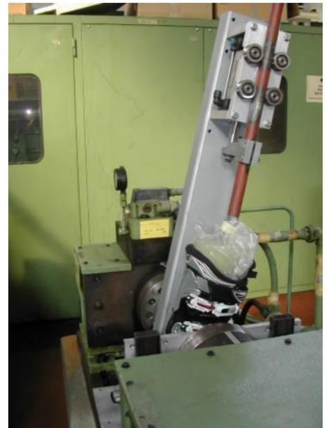
The wheels drive the pole and allow small relative displacements during movement in the direction of the pole axis. The wheels are screwed to the “P-arm” into four holes; two of them have been bored to facilitate the coupling between pole and the four wheels.
