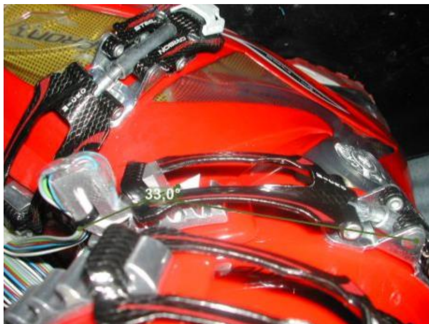
Figure 3. 3 Example of angle measure
