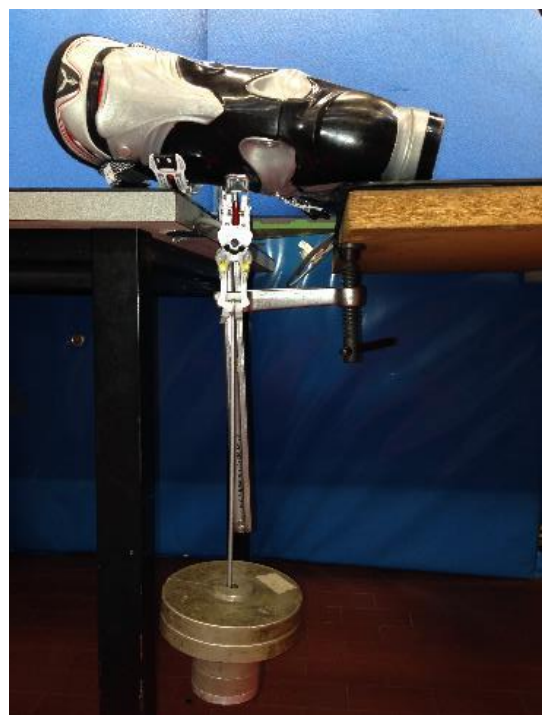
Figure2. 8 Masses application for the buckle calibration
