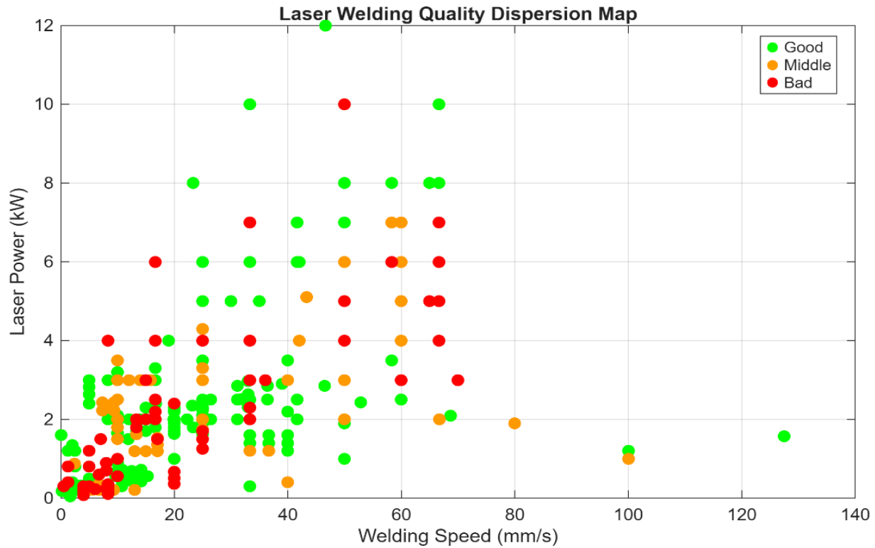
Figure 8. Dispersion Graph shows the relation between Laser Power (KW) and welding speed (mm/s) on weld quality.
