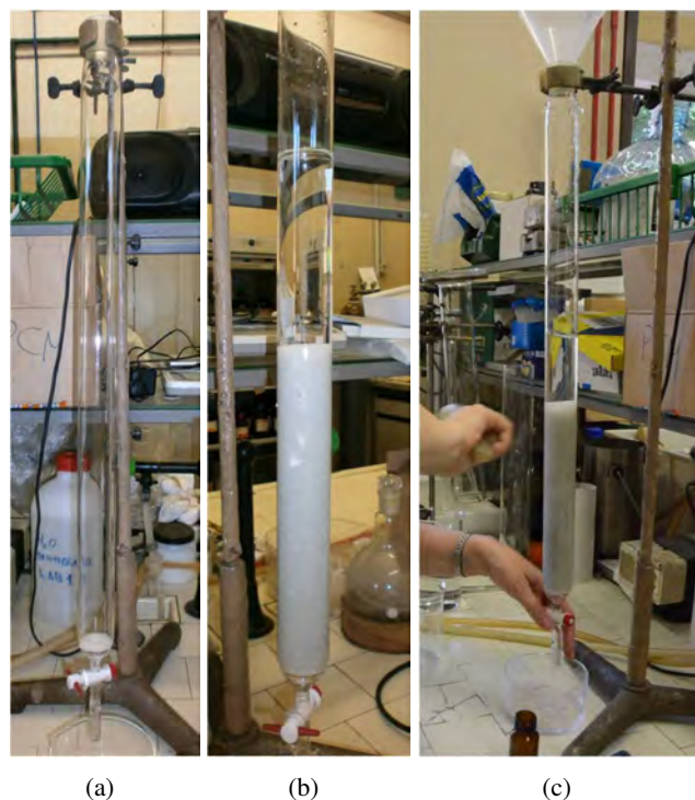
Figure 5.6. Chromatographic column used for the tests (a); saturation of the column (b); compaction of the column (c)
