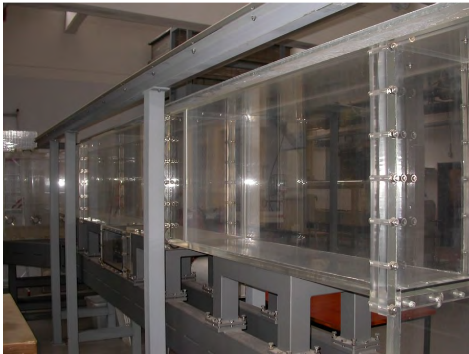
Figure 4.1. Sand-box facility used for the experiment [58]
