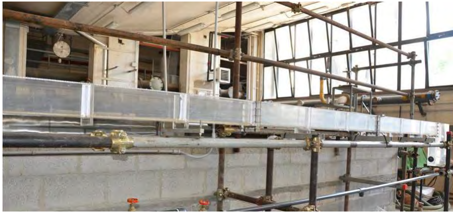
Figure 5.29. Small sand-box device used for the glass beads washing test
