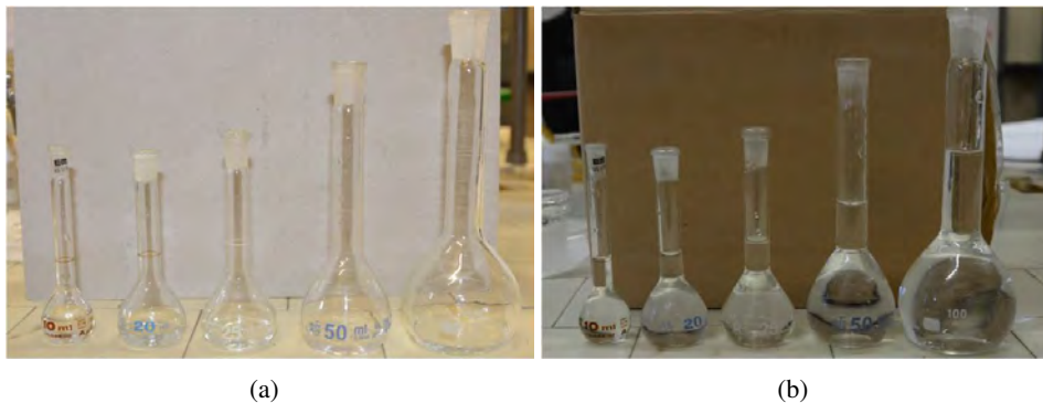
Figure 5.24. Samples diluted with deionized water to obtain the calibration line
