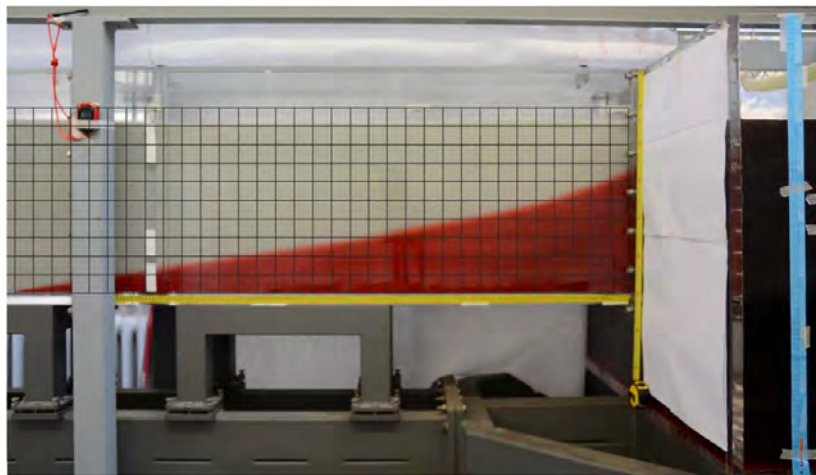
Figure 9.22. Saltwater intrusion after 24 hours
