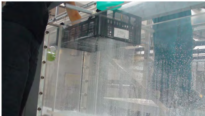
Figure 9.1. Positioning of glass beads in the sand-box device
