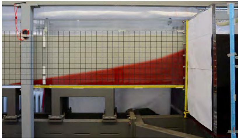
Figure 9.21. Saltwater intrusion after 22 hours
