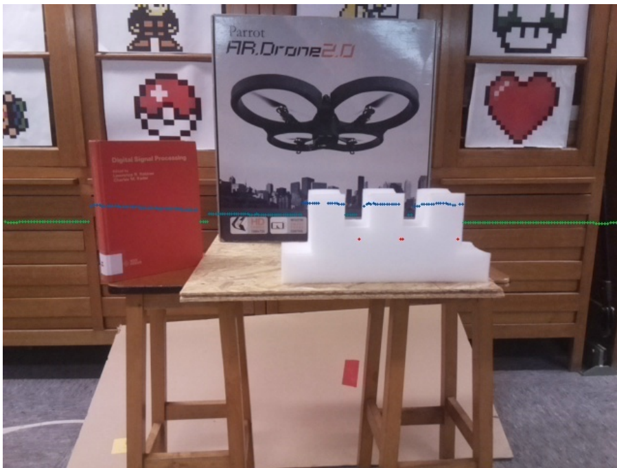
Figure 5.6: exaple of projection of the 2D LiDAR beam over the camera image plane
