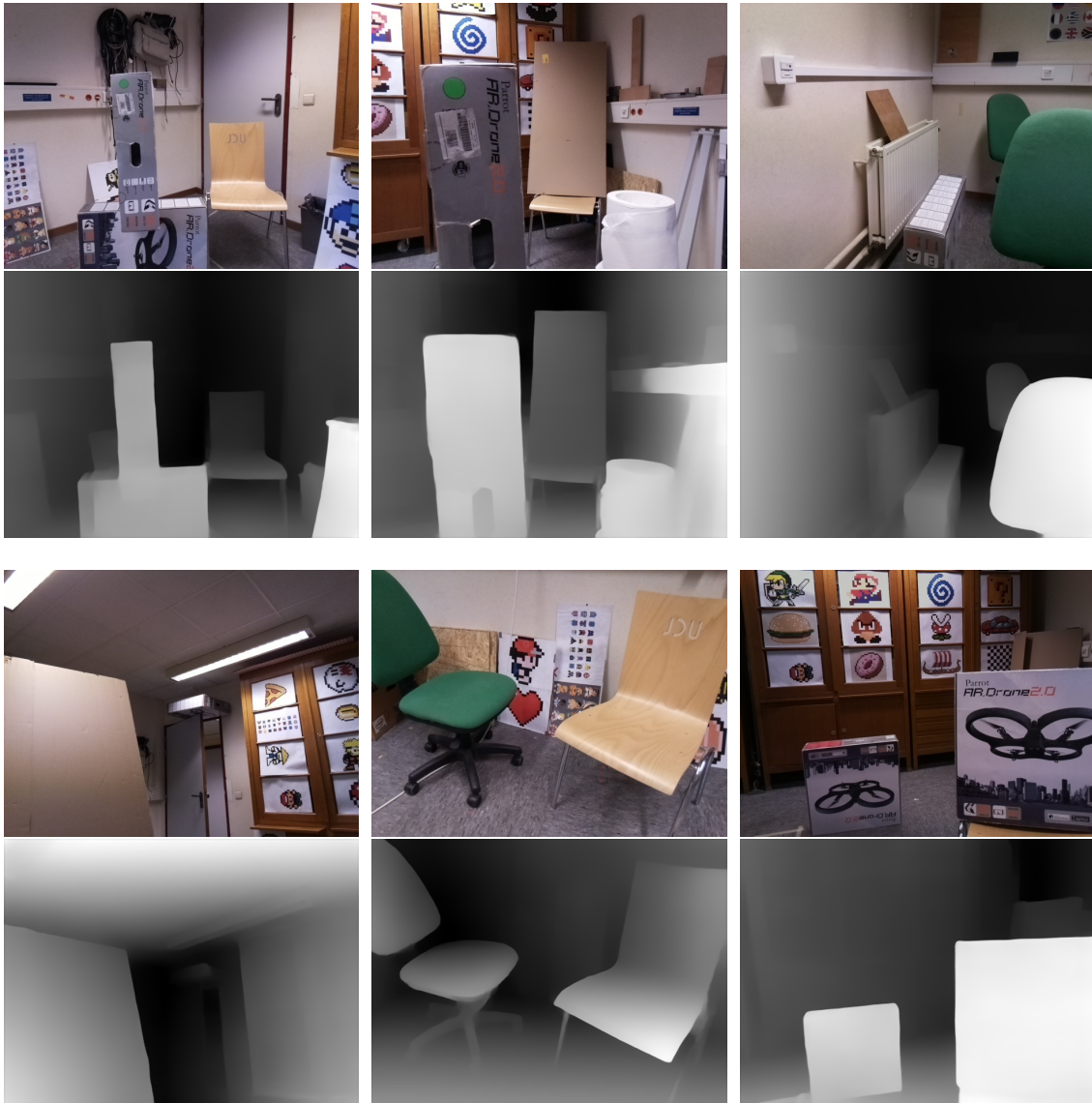
Figure 5.4: examples of MiDaS implementation considering the raspicam V2 camera. The upper part consists into the input image given to the network (in its RGB format), and, in the associated lower part, the processed depth map, obtained ranging the output values from 0 - 255
