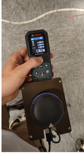
Figure 6.7: example of ground truth annotation through single beam construction LiDAR
