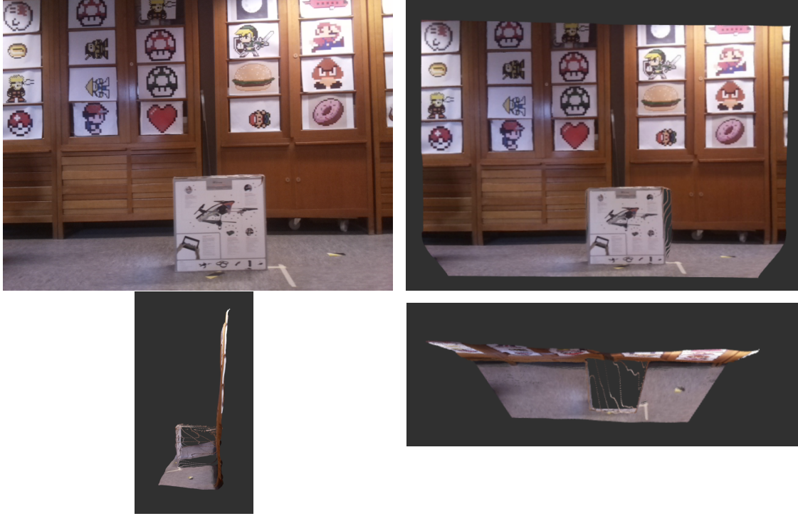
Figure 6.11: From the top-left to the bottom right it is reported: the first scene considered and the obtained pointcloud in terms of its front view, side view and top view
