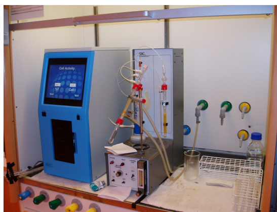
Figure 26 Coulometer used for the analysis, model 5015.
