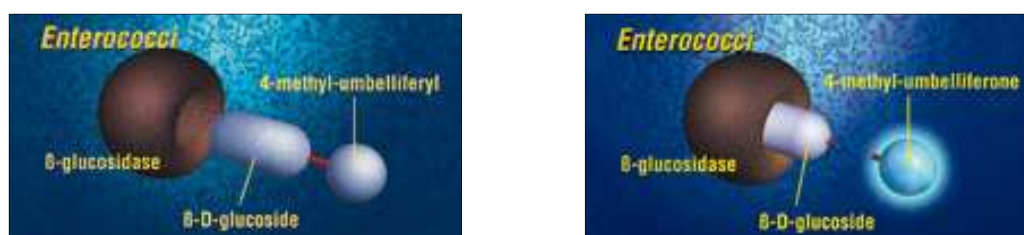
Figure 2.9 Enterolert™ mechanism for Enterococci detection in water
