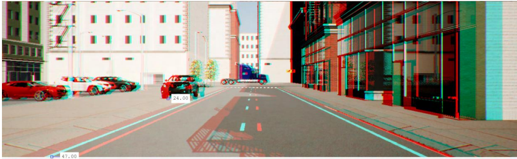
Figure 2.6: Red-cyan anaglyph of the stereo pair in figure 2.4 with the measure of the disparity for two generic points. The road line in the lower left corner was chosen to measure the maximum value, where the distance of coincident points corresponds to 47 pixels.
