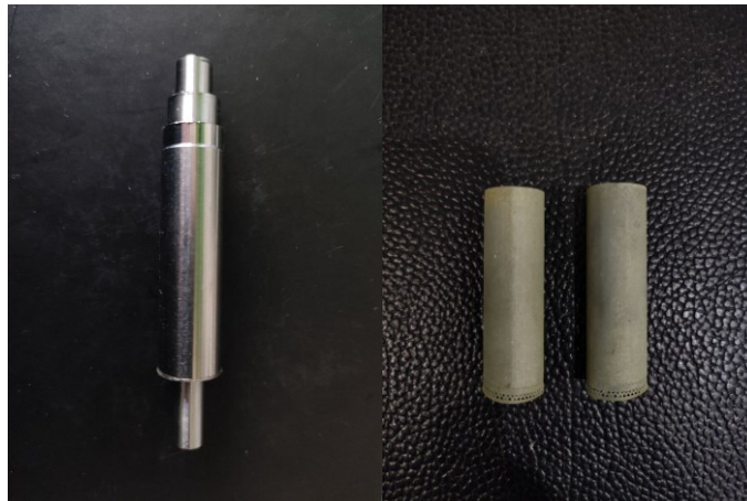
Figure 2.1 One of wrought NiTi bars (left); AM NiTi bars (right)
