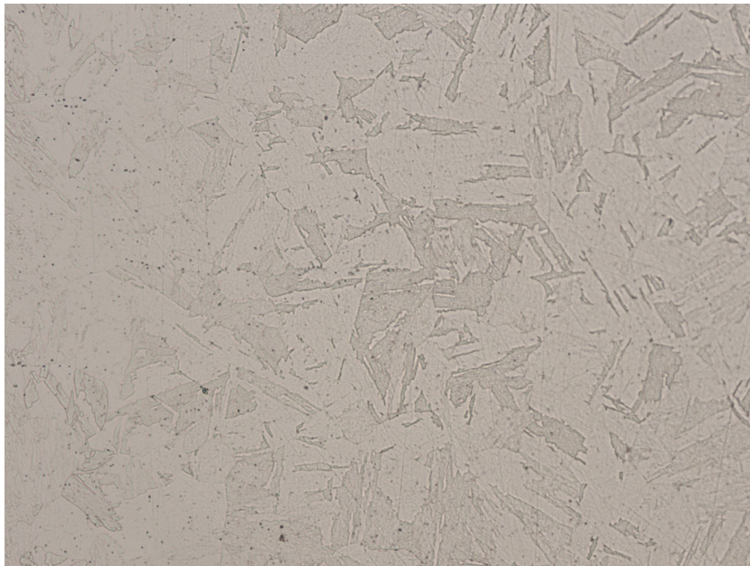
VAR remelted specimen H1100, 500X
