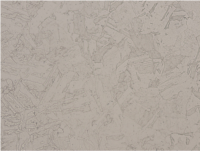
VAR remelted specimen H925, 500X
