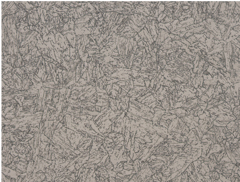
VAR remelted specimen H1150, 500X
