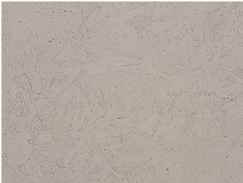
ESR remelted specimen A (solubilized), 500X
