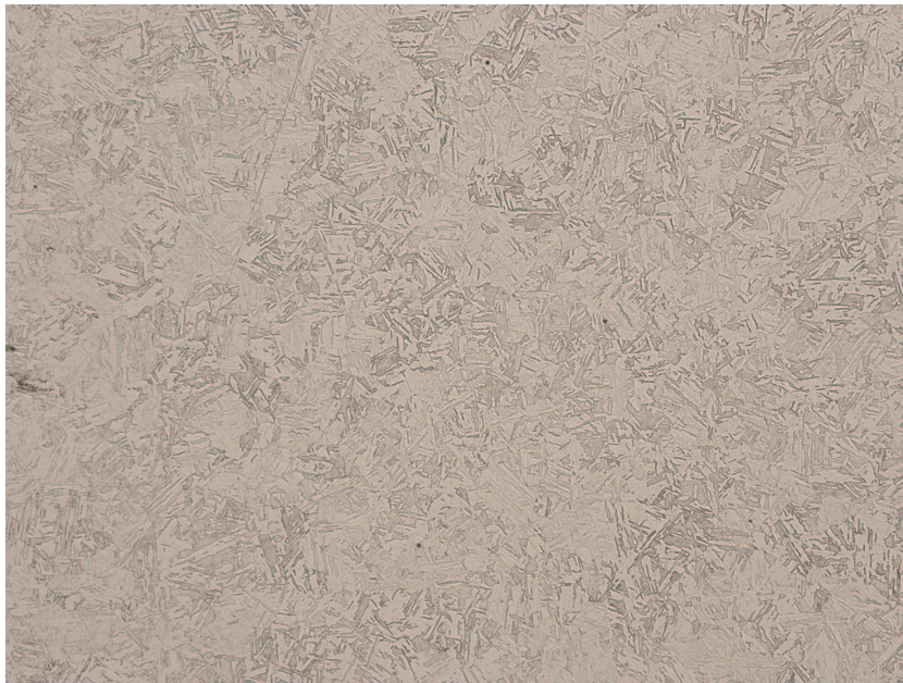
ESR remelted specimen H925, 100X
