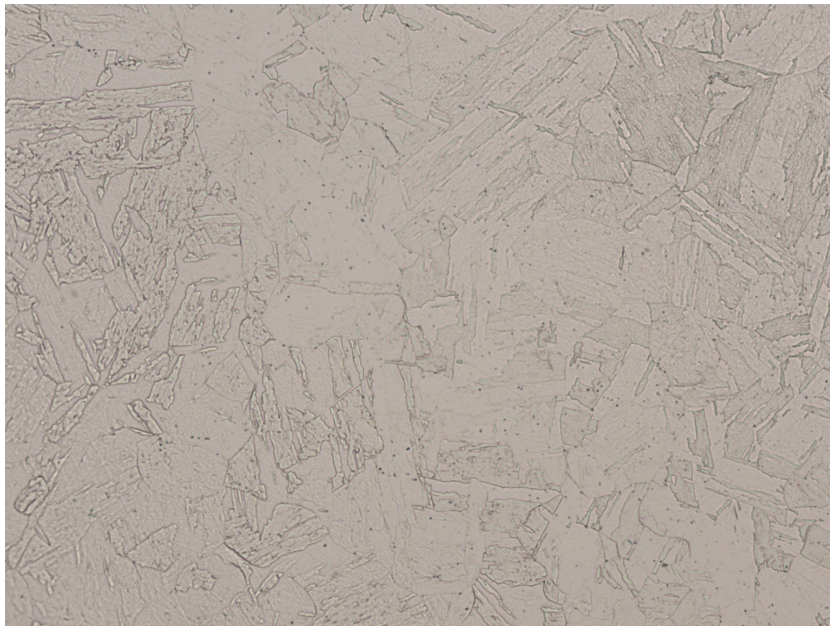
VAR remelted specimen H900, 500X
