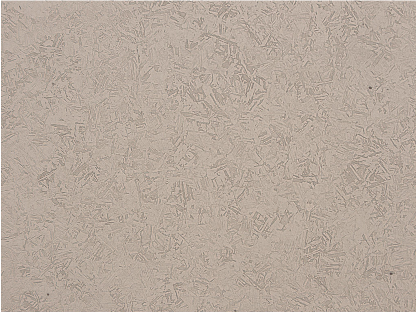
ESR remelted specimen H1025, 100X
