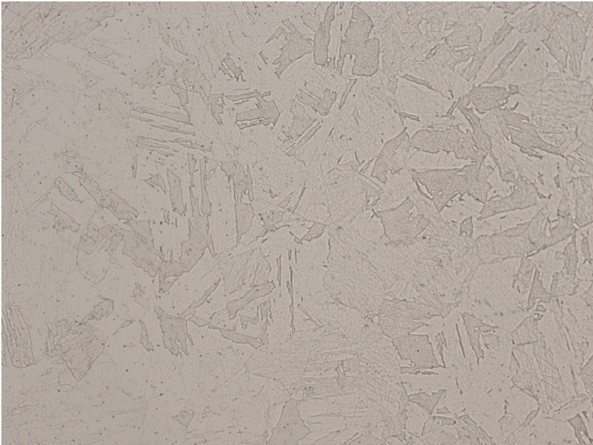
VAR remelted specimen H1075, 500X
