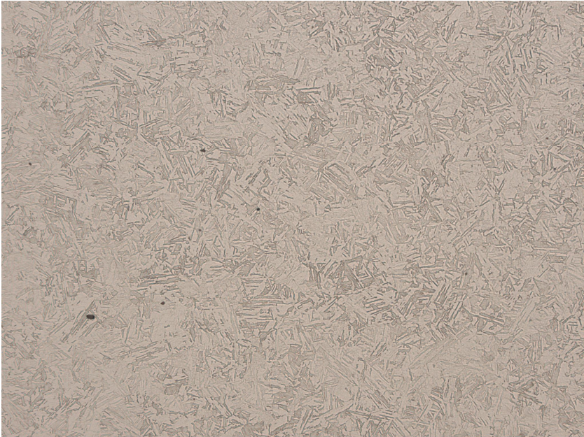
ESR remelted specimen H900, 100X
