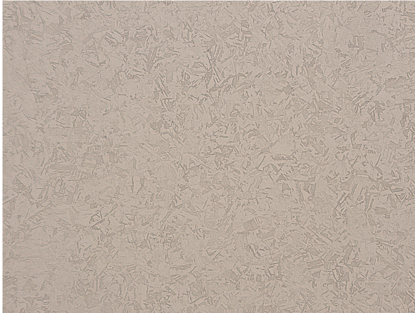
VAR remelted specimen H1100, 100X
