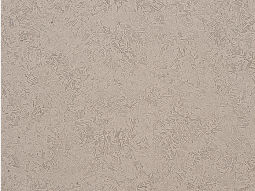
ESR remelted specimen H1100, 100X
