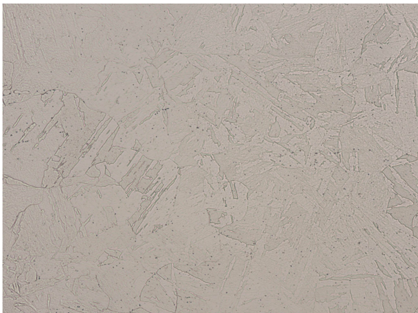
VAR remelted specimen A (solubilized), 500X
