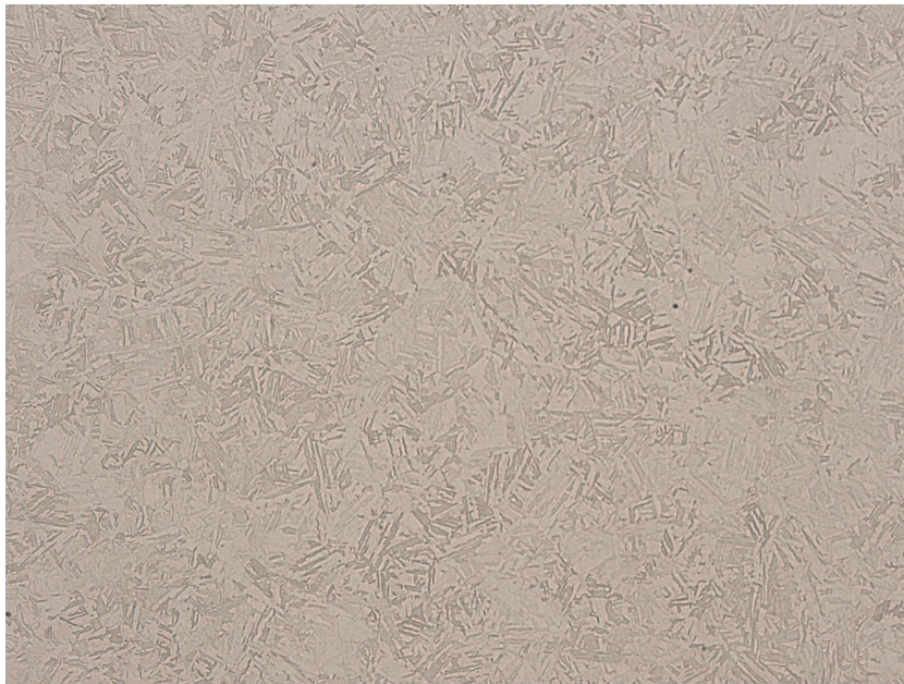
ESR remelted specimen H1075, 100X
