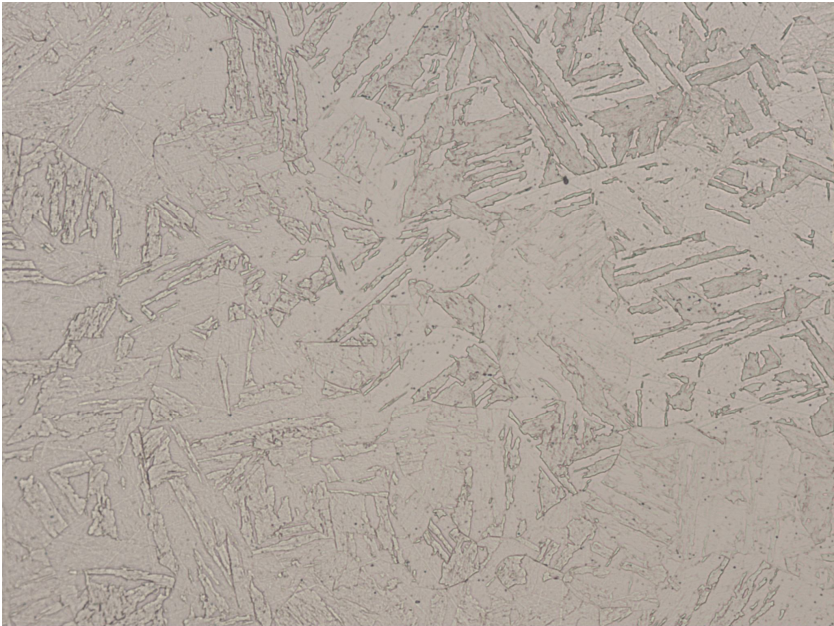
ESR remelted specimen H900, 500X
