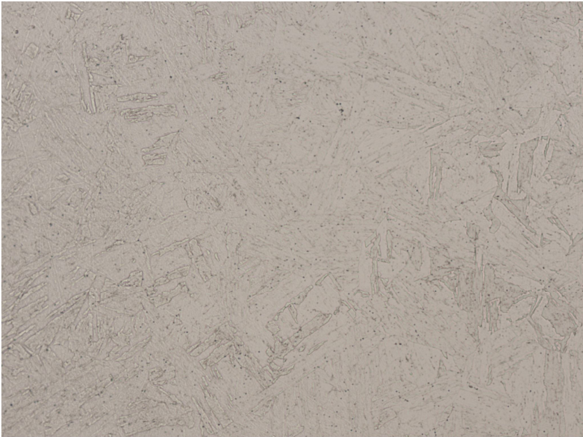
ESR remelted specimen H1100, 500X
