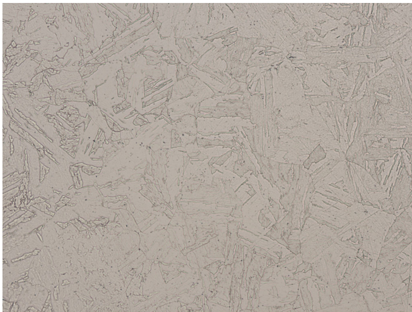
ESR remelted specimen H925, 500X
