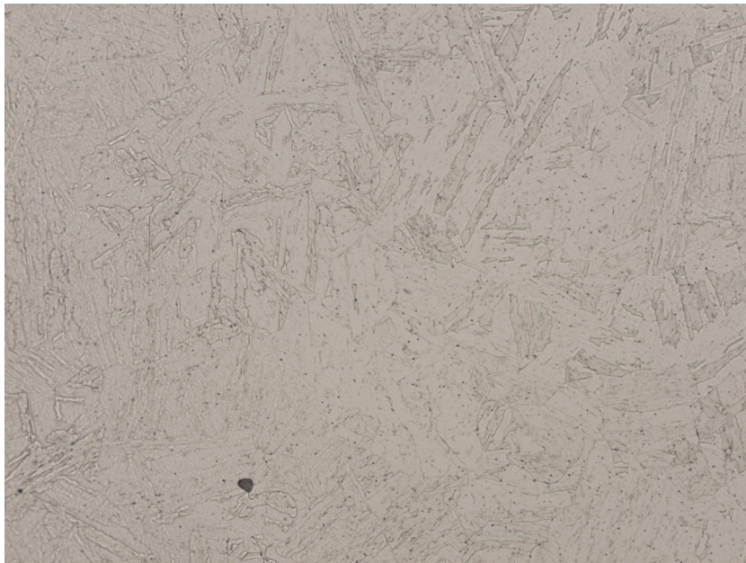
ESR remelted specimen H1075, 500X
