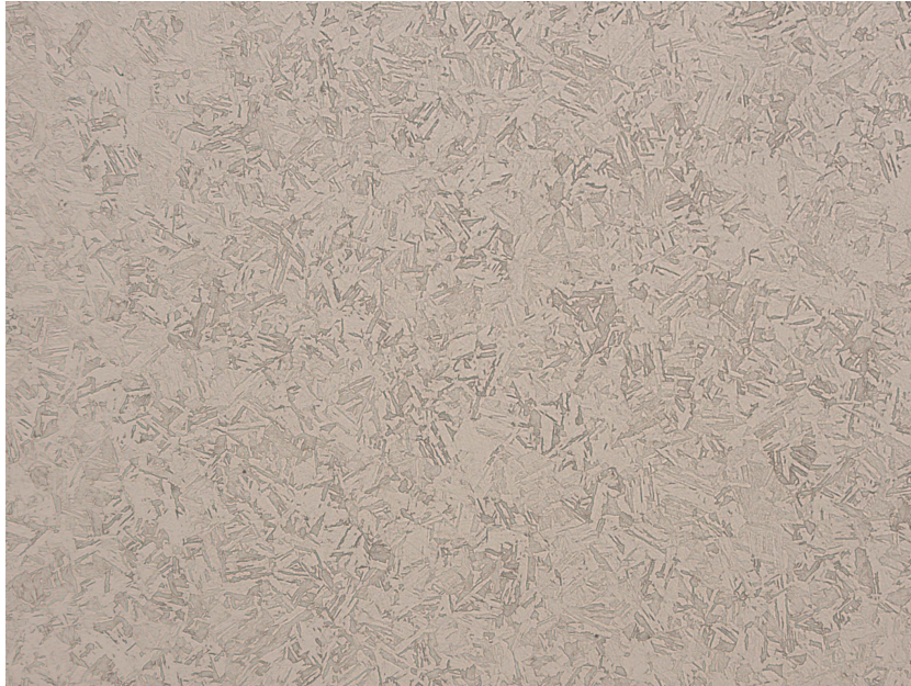
VAR remelted specimen H900, 100X
