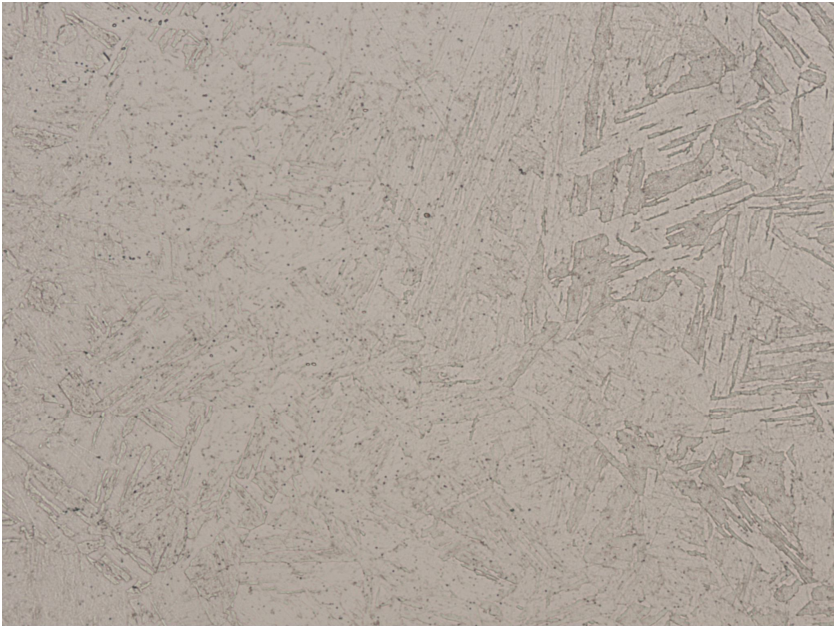
ESR remelted specimen H1025, 500X
