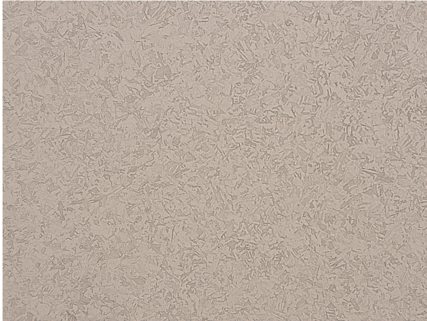
VAR remelted specimen H1025, 100X
