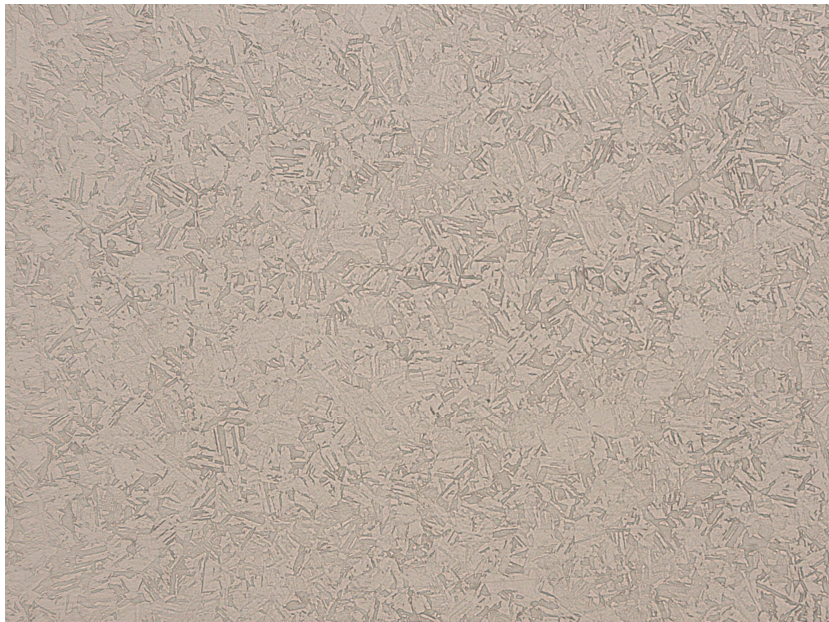
VAR remelted specimen A (solubilized), 100X
