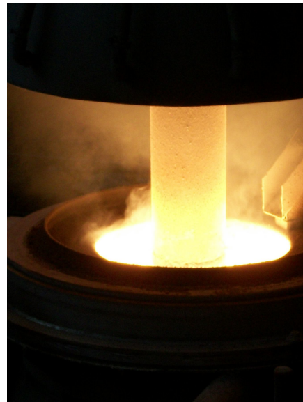
Fig. 5.16 Schematic of electroslag remelting, and the insertion of the electrode into the slag.
