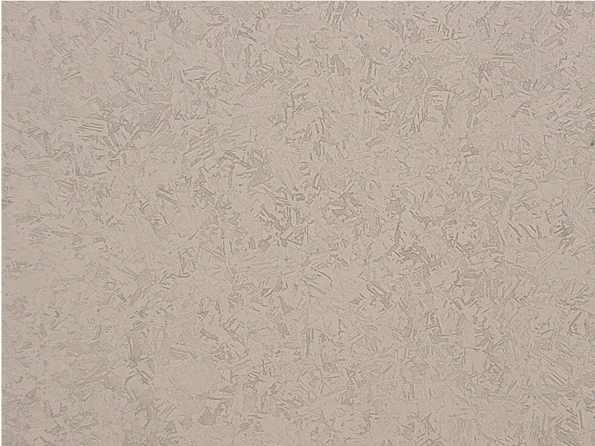
VAR remelted specimen H1075, 100X
