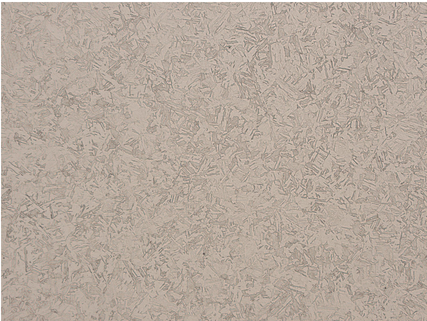
VAR remelted specimen H925, 100X
