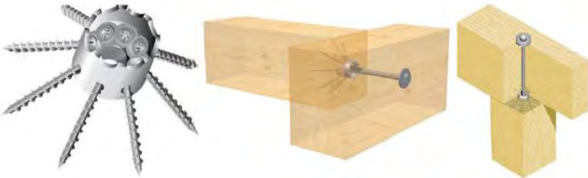
Figure 2.11 Sihga Idefix innovative connection systems (Sihga)
