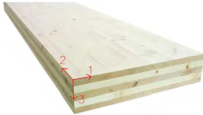
Figure 4.1 Orientation of local axes in a generic X-Lam panel
