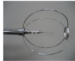
Figure 15 Close view of the anemometer Sensoanemo.
