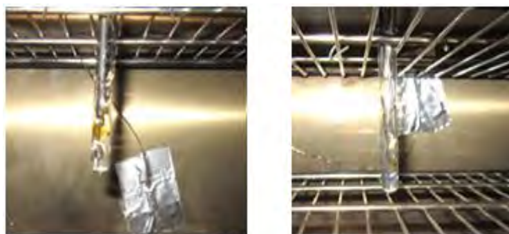
Figure 3.10 Melting of polyethylene samples at 220°C in oxidizing atmosphere (left) and inert (right).
