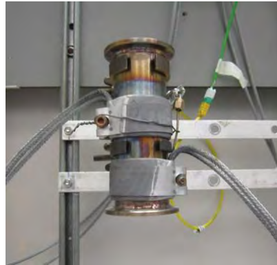
Figure 6.20 Second resistances and pliers' configuration along the reactor.
