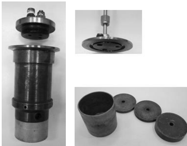
Figure 6.1 Kettle-type reactor with screw (left) cap, flat cap and inner configuration (right).
