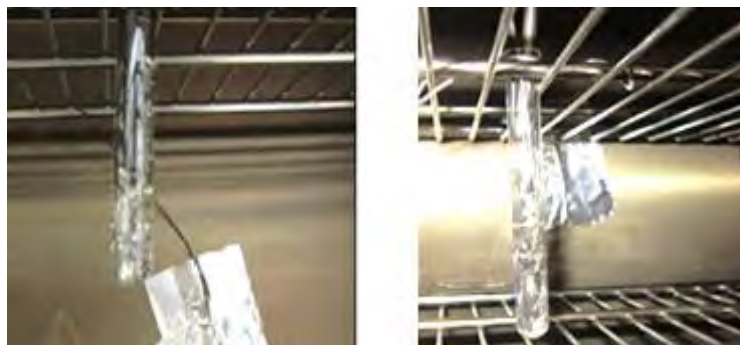
Figure 3.9 Melting of polyethylene samples at 170°C in oxidizing atmosphere (left) and inert (right).
