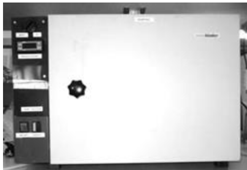
Figure 3.1 Laboratory oven equipped with PID regulation.
