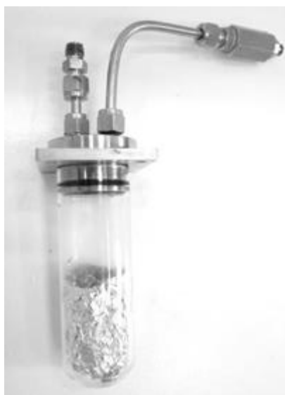
Figure 6.29 Condenser test tube without pipe and with aluminum paper inside.
