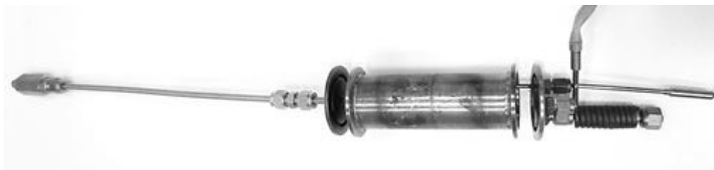
Figure 6.5 Tubular reactor with covers, control thermocouple and tubular resistance.
