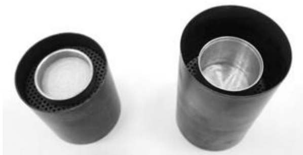
Figure 6.28 Different size crucibles and hollow cylinders to hold them.
