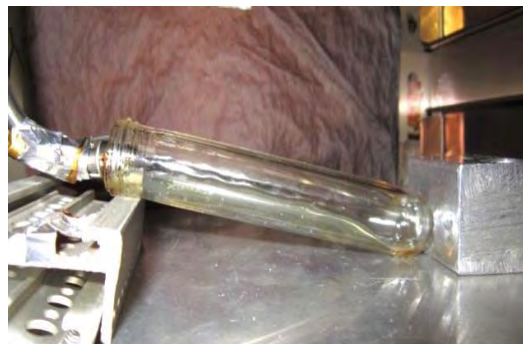
Figure 3.14 Polyethylene after 160 minutes at 240°C in 70 ml/min of Argon flux.
