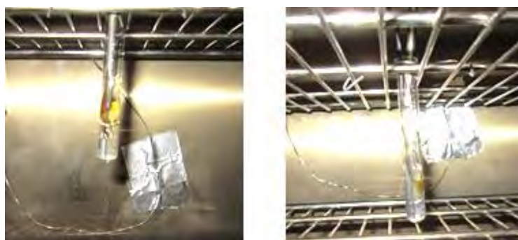
Figure 3.11 Polyethylene samples after 20 minutes at 220°C in oxidizing atmosphere (left) and inert (right).
