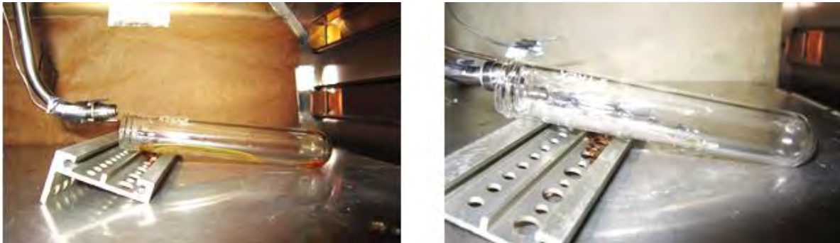
Figure 3.13 Polyethylene samples after 40 minutes at 180°C in oxidizing atmosphere (left) and inert (right).
