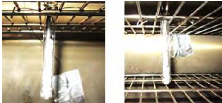
Figure 3.8 Test tube placed in the oven holding polyethylene in oxidizing atmosphere (left) and inert (right).
