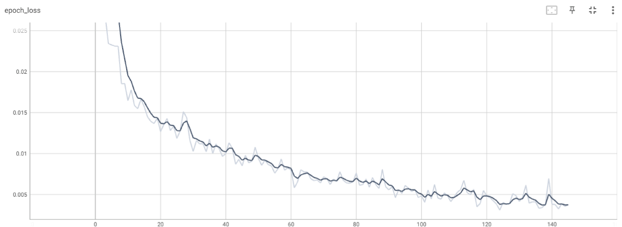
Figure 6.12: Epoch - loss graph when the learning rate is set to 1e-3 on TensorBoard.
