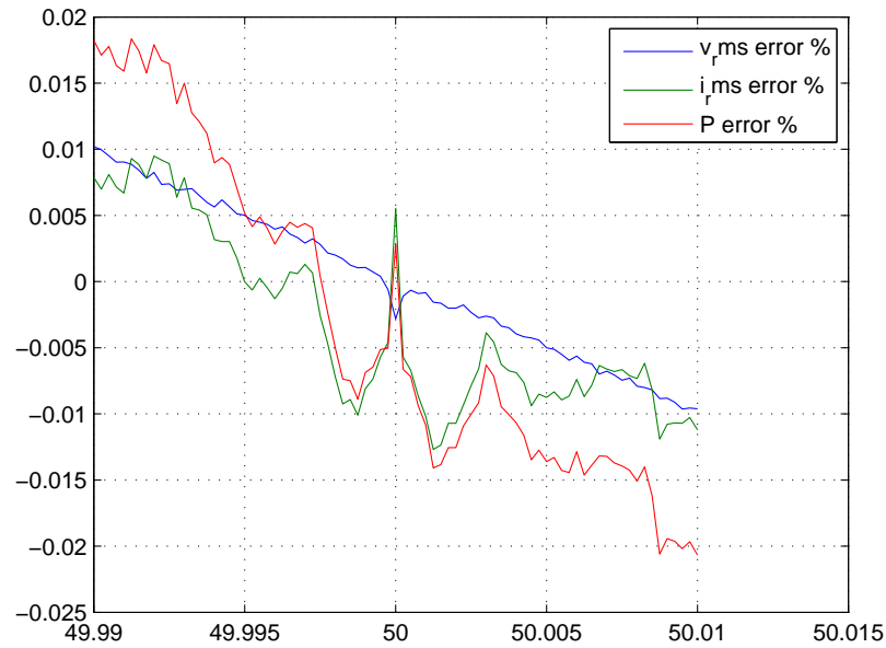
Figure 6.6: Errors in the evaluation of V_{rms} , I_{rms} and P due to non synchronized sampling with a 10 cycles window and a current of 10% of the full scale
