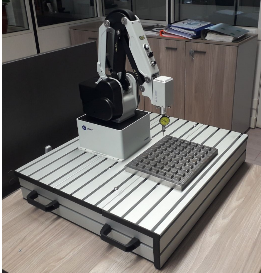
Figure 2.6: Photo of the experimental setup for the test phase using the comparator and milled aluminum plate.
