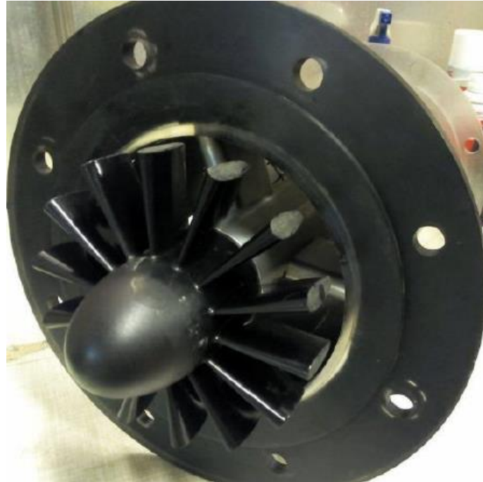
Figure 3-3 Fan simulator used by Cranfield University in the experiments [8].
