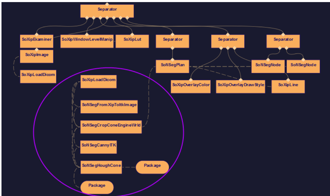
Fig. 7.10: Scenograph of the needle detection algorithm by means of Hough transform and highlighted by the purple circle. The rest of the scene graph refers to a simulation of the planning step, in order to provide entry and target point.
