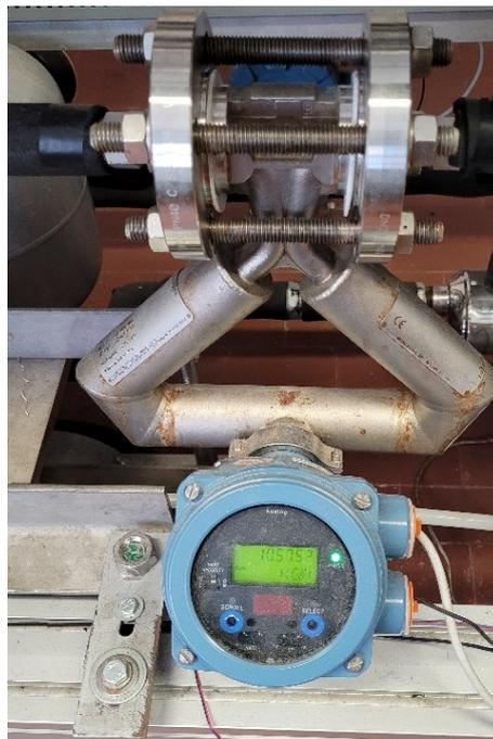
**Figure 2.4.** Coriolis flowmeter.
