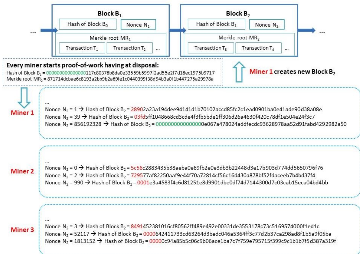
Figure 25 - An example of the nonce mechanism for the proof-of-work Source: Personal elaboration
