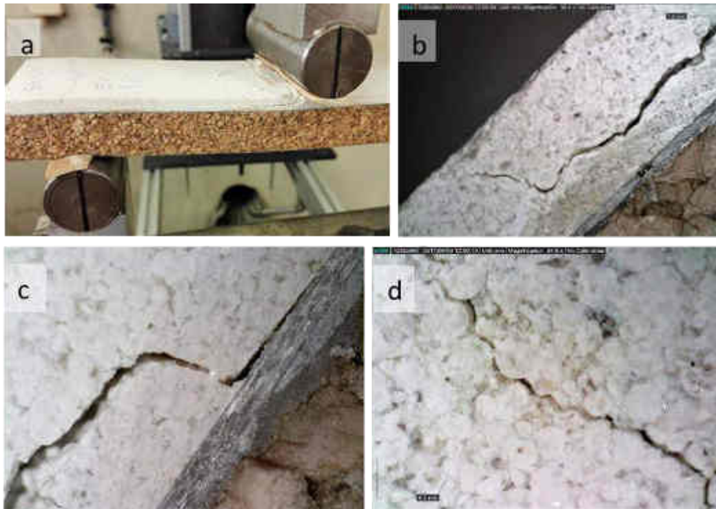
Figure 5.3 Macrocrack propagating below roller contact parallelly to the resin-rich layer; b) Crack kinking upwards in phase V; c) Crack kinking downwards in phase V and causing delamination; d) Evidence of intergranular fracture propagation
