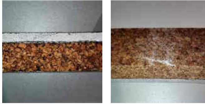
Figure 5.20 Specimen tested at 60% with resting time. Left: crack on the stone. Right: whiting of the resin.
