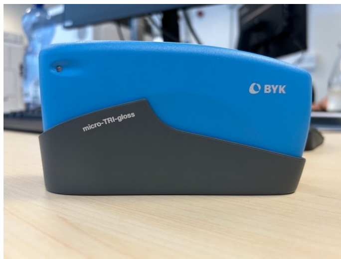
Figure 6. 4: Micro-TRI-gloss BYK. It allows a measure of the gloss value at 20°, 60° and 85° simultaneously.
