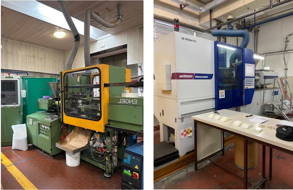
Figure 6. 3: Injection molding machines. On the left Engel ES150/50 , present in R&D lab, on the right Wittman Battenfeld Ecopower 55/130 , present in QC lab.
