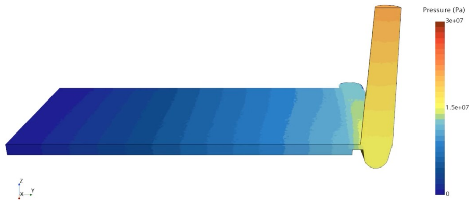
Figure 7. 61: Pressure profile in QC mold filling. The color scale indicates the intensity of pressure: blue correspond to zero and red to the maximum pressure.
