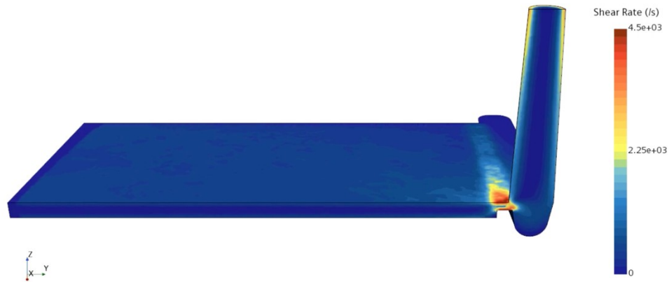
Figure 7. 59: Shear rate profile in QC mold filling. The color scale indicates the intensity of shear rate: blue corresponds to zero and red corresponds to the maximum shear rate.
