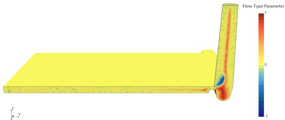
Figure 7. 57: Flow type behaviors in QC mold filling. The color scale indicates the type of flow: red represents pure elongational flow, yellow represents pure shear flow and blue rotational flow.
