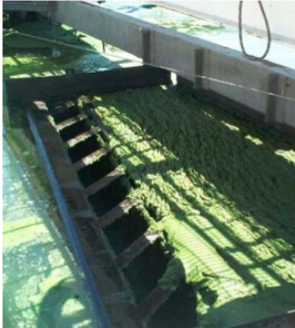
Fig. 17. Chemical coagulation plus flotation (Lundquist, 2008).
