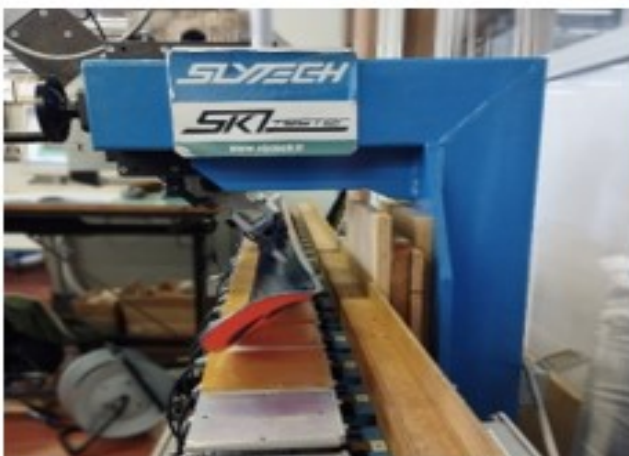
Figure 2.7: Slytech test bench in use and detail of rocking plates
