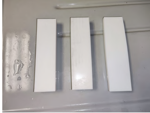
Figure 4.10: PTFE moulds after the compression. Those in the center and on the right, respectively at 100 and 200 bar, appear deformed compared to the one on the left where manual pressure was applied.
