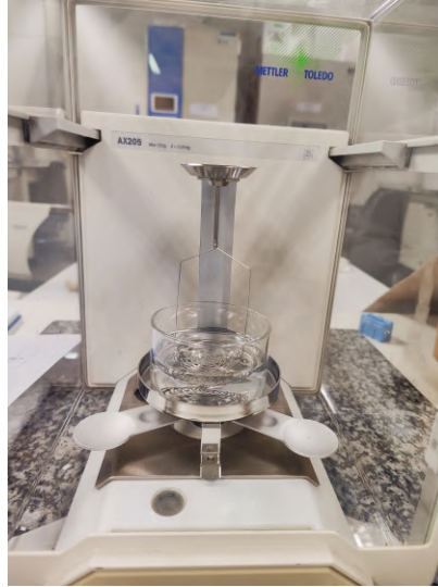
Figure 3.13: Hydrostatic scale. The weight is placed in the submerged grid, while at the top the sample can be weighed before submerging it and then the weight can be calibrated
