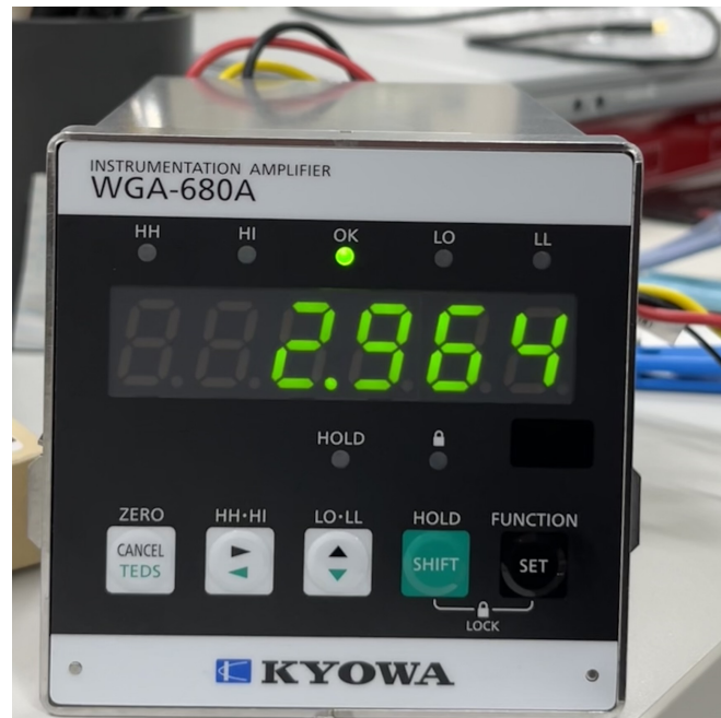
Figure 3.11: Actual force measured in steady-state with a force sensor located on the back of the motor tip.
