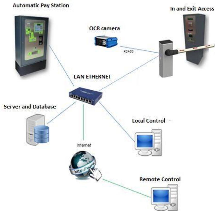
Figure 1 The proposed system architecture
