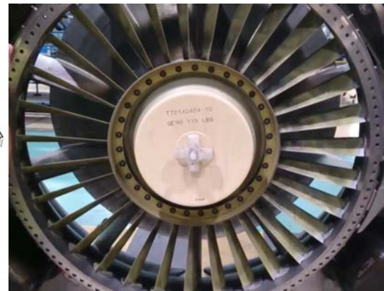
Figura 1.7: GE90-115 Inlet Guide Vanes mobili
