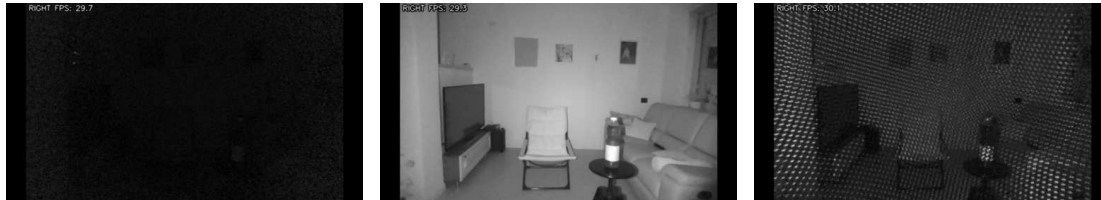
(a) Environment with low light conditions (b) Flood illumination active (c) IR dot grid active
