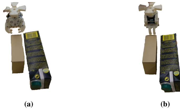
Fig. 5.4: Possible pushing poses to push an object along its principal axis: In Figure (a) the closing direction of the gripper is orthogonal to the pushing direction, and for the case depicted in the figure the gripper would likely push also the black juice box. In Figure (b) the closing direction of the gripper is parallel to the pushing direction.
