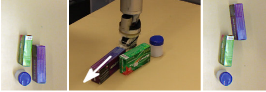
Fig. 3.2: The pushing length l is function of the neighbour objects. The first image shows the configuration before moving the purple box. The second one shows the execution of pushing the purple box. In the third one we see the purple box is moved to a graspable pose.
