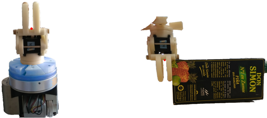
Fig. 5.2: The gripper and its base. Fig. 5.3: Profile view of a desired pose for pushing an object.
