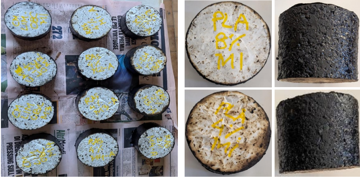
Figure 3.12(b): Compacted samples from Suprapave gyratory compactor
