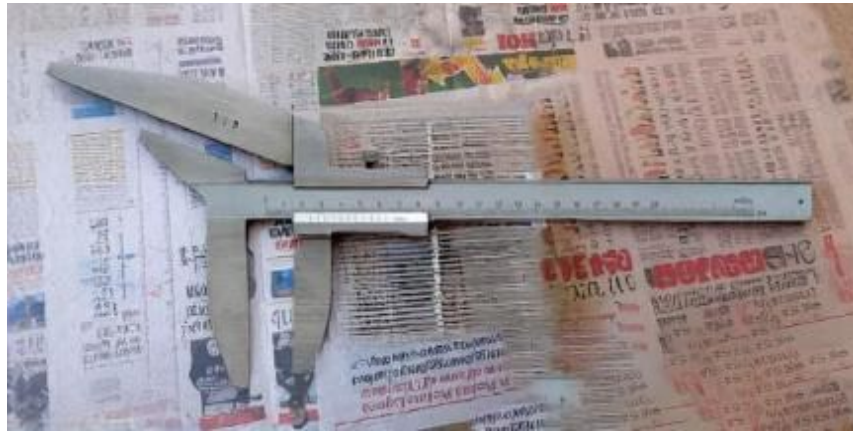
Figure 3.8: Grain size caliper used for Shape Index
