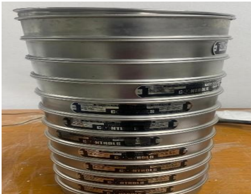
Figure 3.4: Sieving of aggregates to determine particle size distribution.
