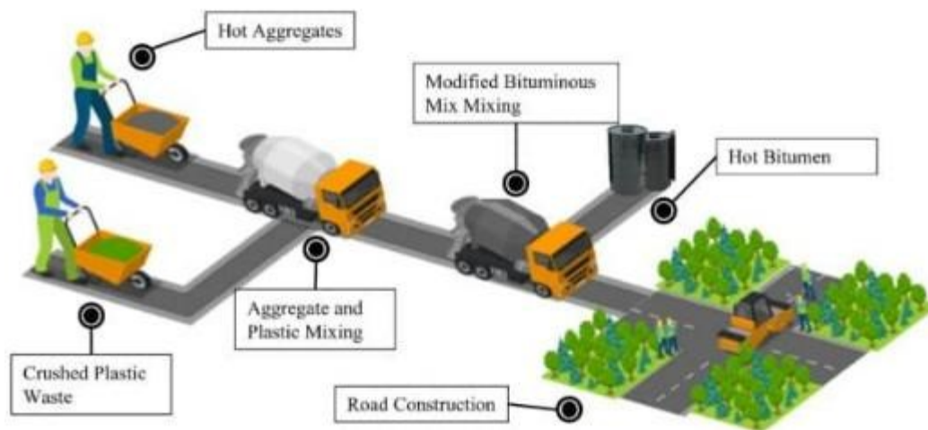
Figure 2.2: The dry process scheme. [3]
