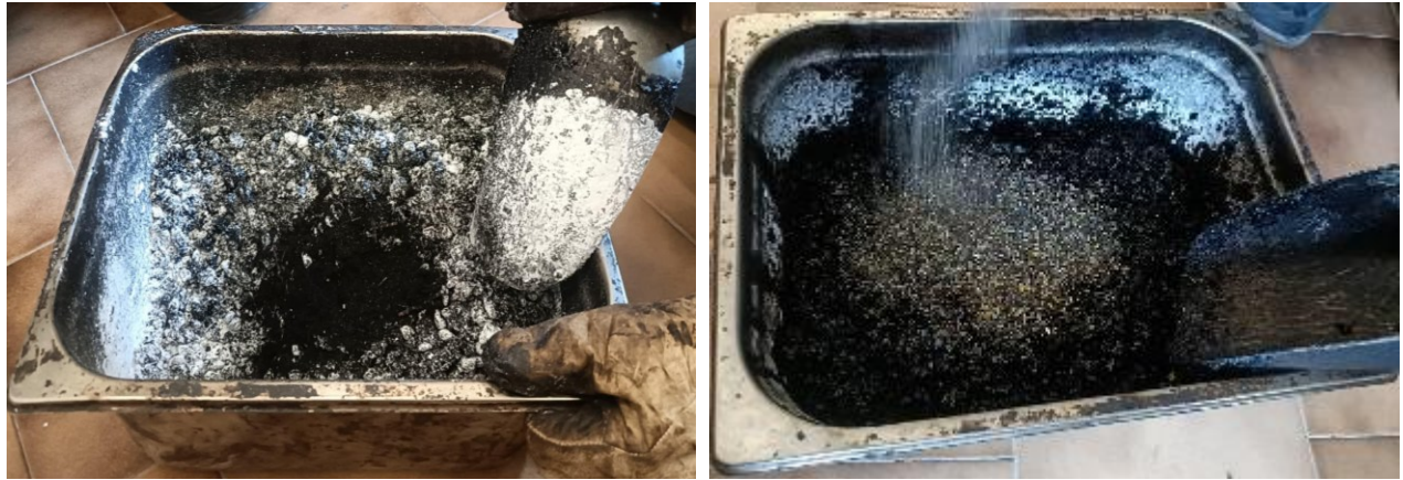
Figure 3.11: Sample mixing using the dry method
