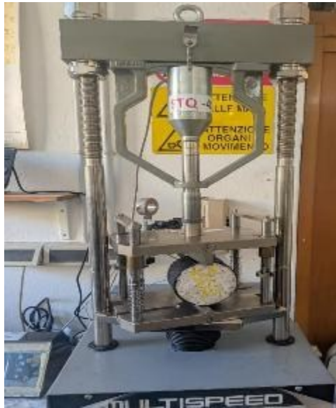
Figure 3.15: Experimental setup for Indirect Tensile Strength (ITS).
