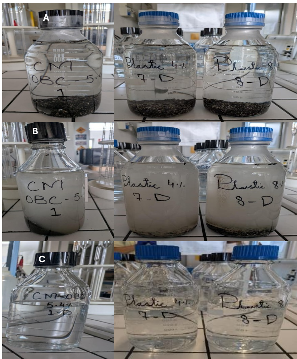
Figure 5.1: (A) Prepared samples before agitation (B) Samples after 24 hr of agitation (C) Leachate after vacuum filtration
