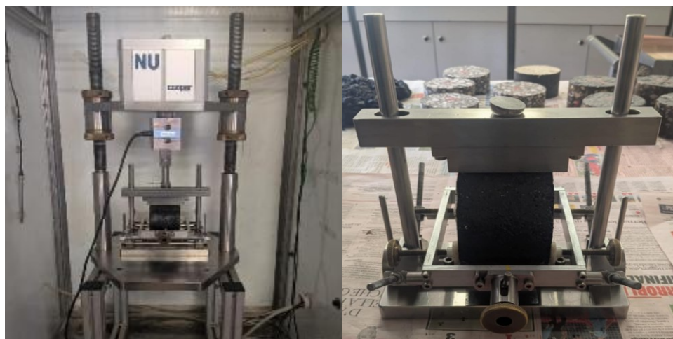
Figure 3.14: Indirect Tensile Stiffness Modulus (ITSM) testing of an asphalt specimen.
