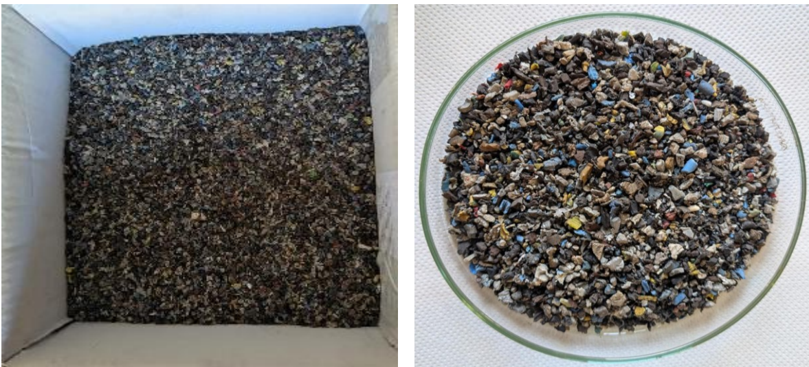
Figure 3.3: Shredded cable insulation waste used in this study.
