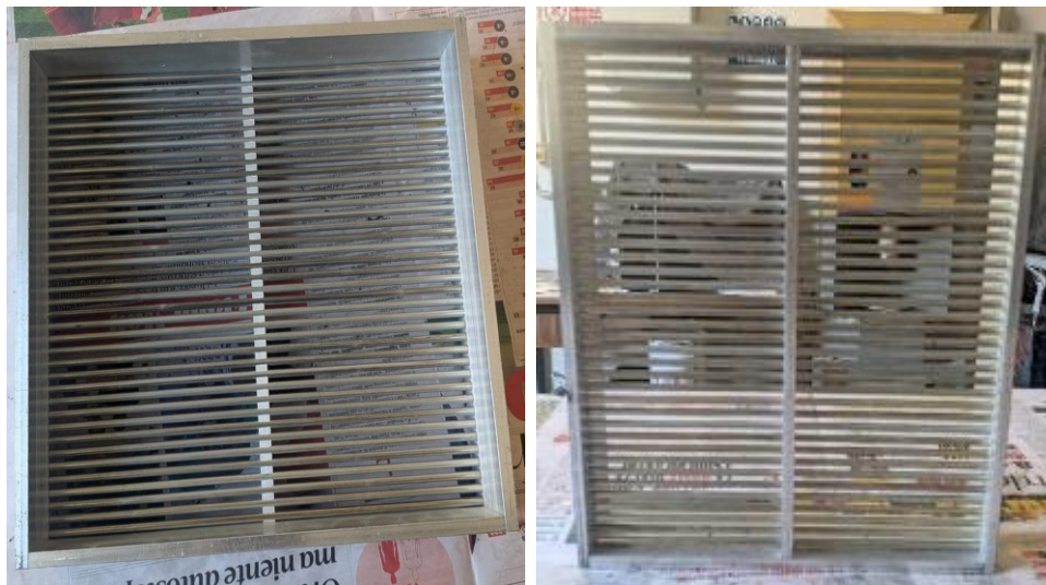
Figure 3.7: Bar Sieves used for Flakiness Index
