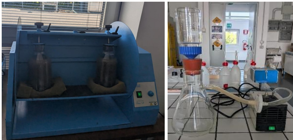
Figure 5.2: Experimental setup for the leaching test, including the laboratory shaker and vacuum filtration apparatus.
