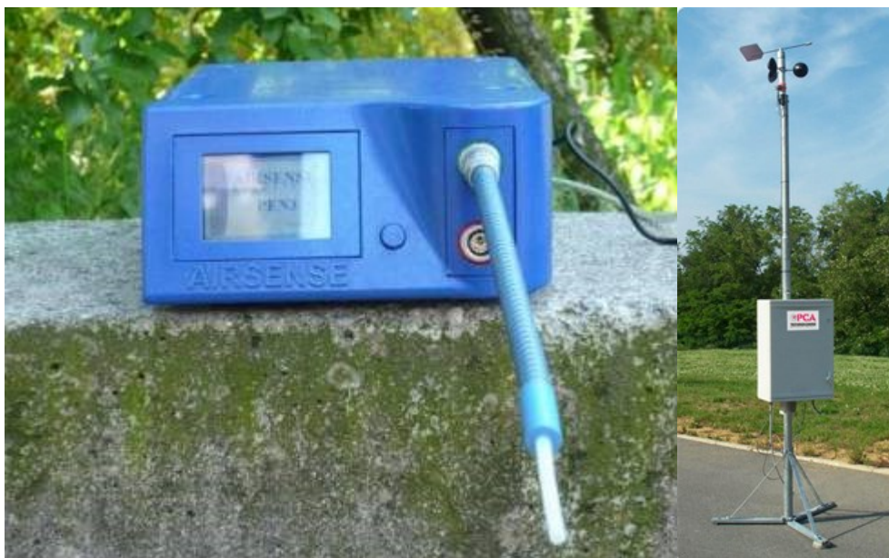
Fig. 5.4 Pictures of the sensory analyzer ("electronic nose") used in the olfactometric survey
