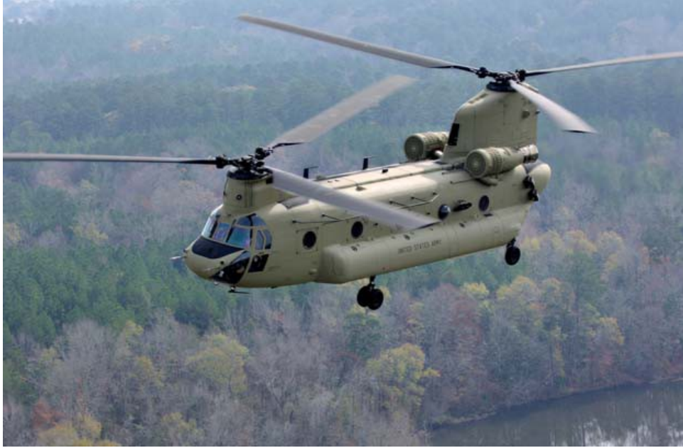
Figure 1.3 A tandem helicopter: CH-47 Chinook [9]
