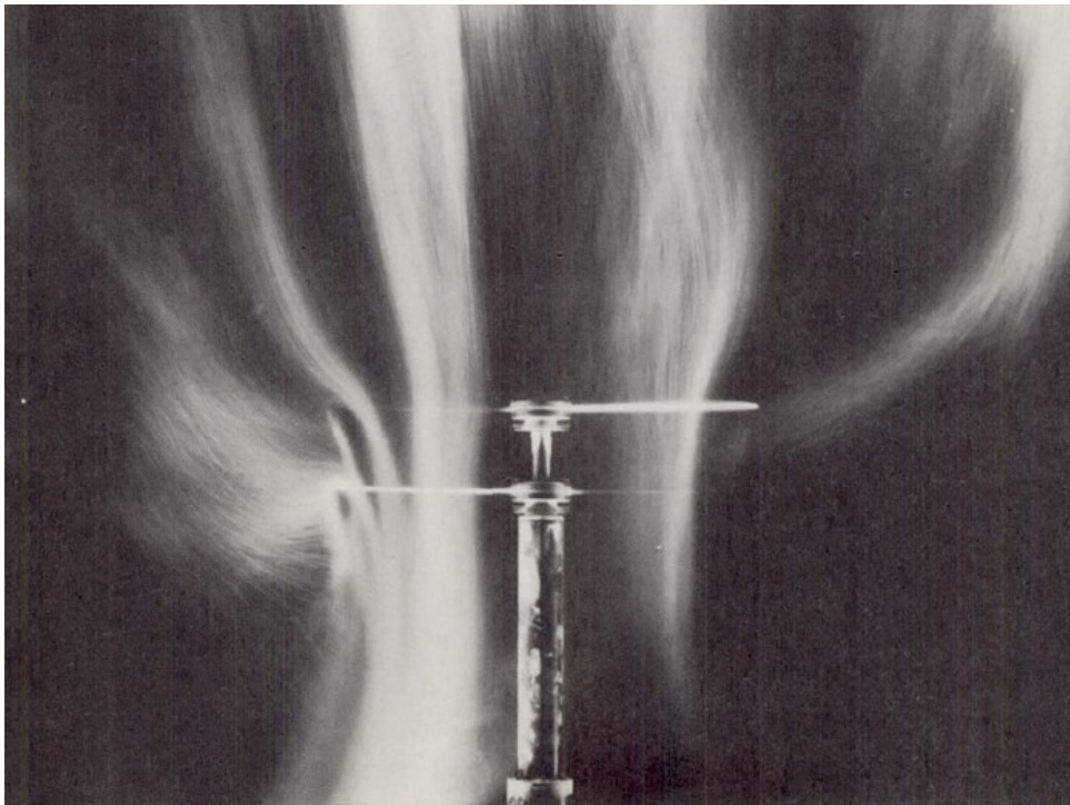
Figure 3.8 Air flow through a coaxial rotor model in static thrust ([28], pag. 8, fig. 2)
