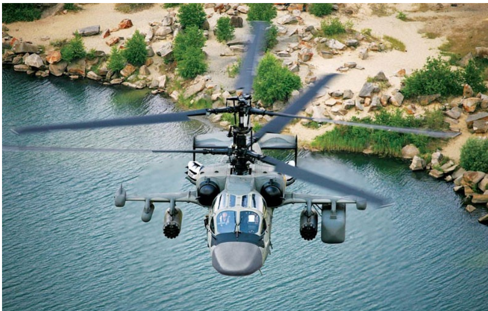
Figure 1.2 A coaxial helicopter: the Kamov Ka-52 Alligator attack helicopter [7]
