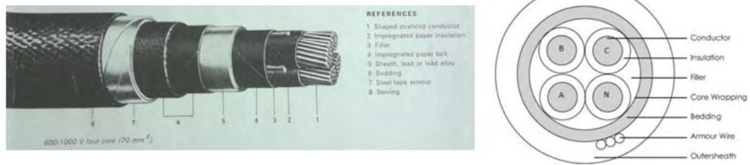
Figure 2.10 PILCSTA underground cable [4]
