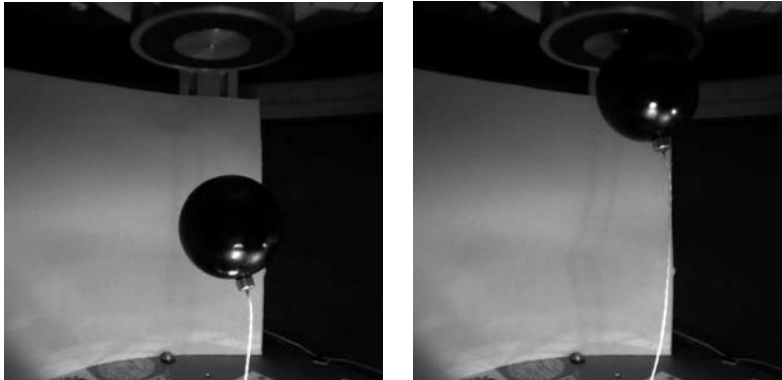
Figure 4.1: Probe's approach to the electromagnet and consequent docking.
