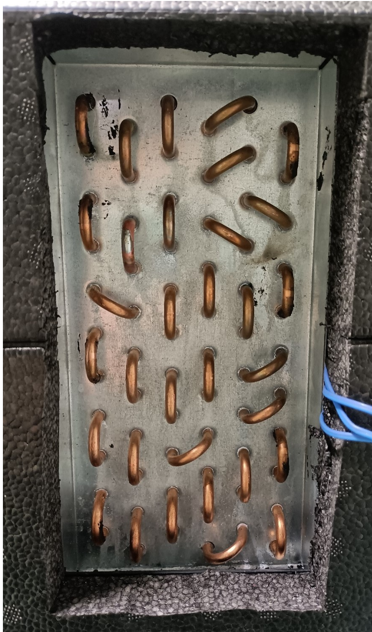
Figure 87: Source heat exchanger view
