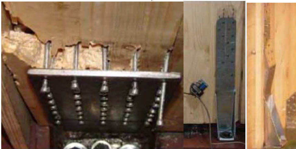
Figura 4.67: Rotture fragili hold-down. Immagini tratte da dispensa lezioni e da "Capacity seismic design of X-Lam wall systems based on connection mechanical properties" Gavric et al. 2013.
