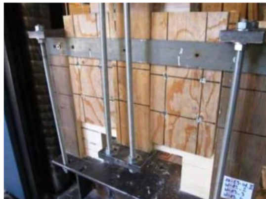
Figura 4.69: Test su giunto verticale. Immagine tratta "Experimental cyclic tests on cross-laminated timber panels and typical connections" Gavric et al. 2013.
