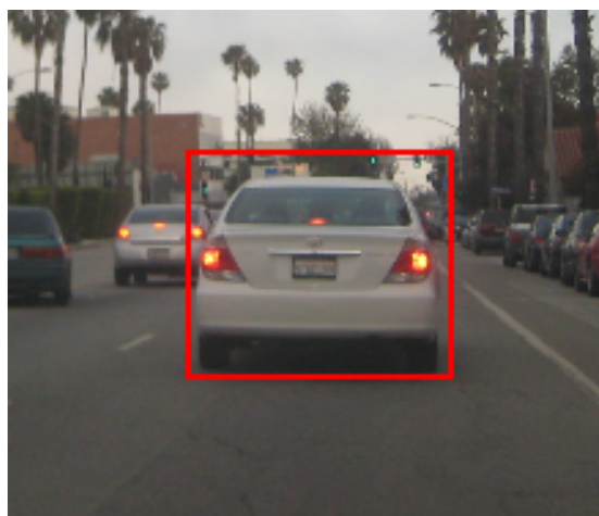
Figure 4.9: Annotation detail - Detail of the annotation used by our application using bounding boxes: the box surrounds the object avoiding to occlude other neighbor objects.
