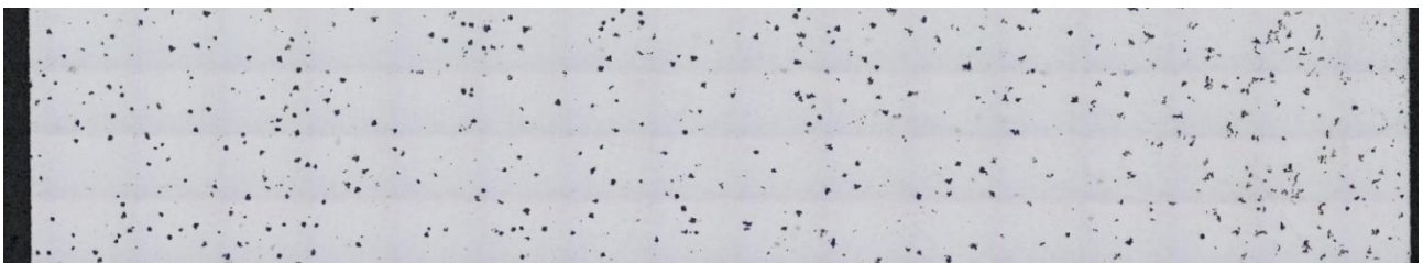
Figure 53 : Optical microscope figure at 5x of the general view of the X2 sample used for the graphite quantification.
