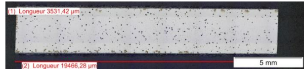
Figure 71 : Optical microscope figure at 2.5x of the general view of the XD2 dilatometer sample.
