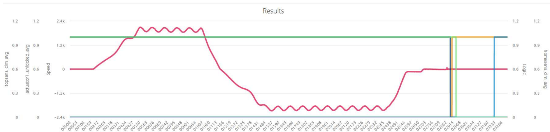
Figure 3.20: Actuator1Locked (—), Actuator1Unlocked (—), TopsensCIm (—), HomesensCIm (—), DrActualspeedRpm (—). Cycle 0026 type 1A, November 19th.
