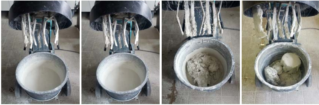
Figure 5.2: Steps in the mixing procedure used to prepare the soil mixture samples.
