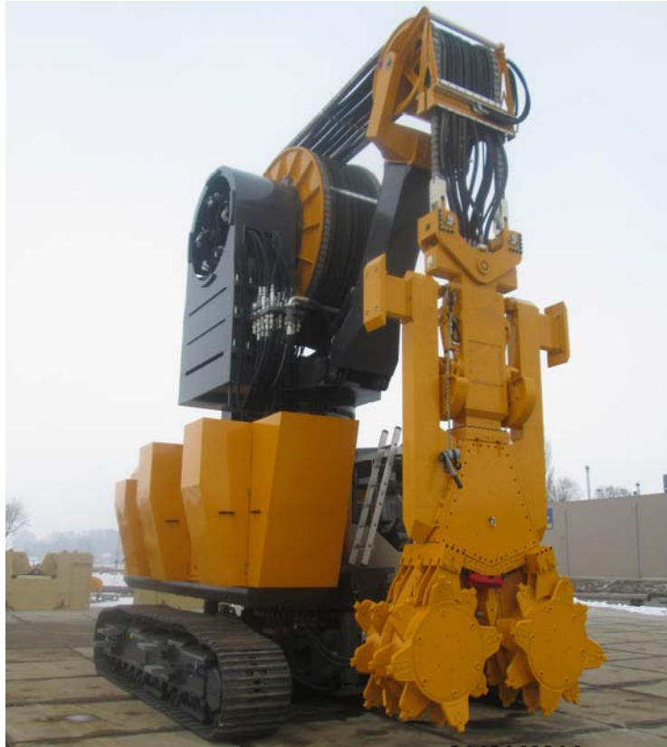
Figure 4.2: CSM (Cutter Soil Mixing) equipment mounted on freely suspended system (Courtesy of BAUER Group).
