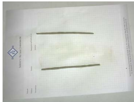
Figure 5.7: Plastic limit test showing bentonite rods.
