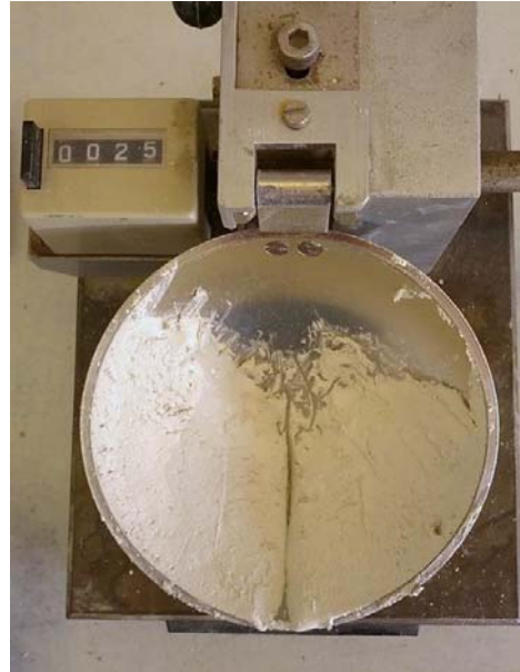
Figure 5.6: Casagrande spoon with illite at its liquid limit.
