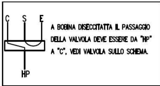
Figura 6-30: Schema valvola a 4 vie.
