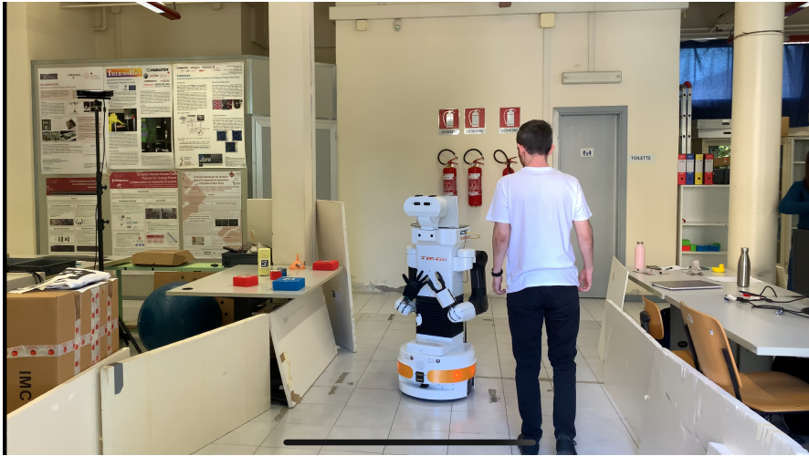
Figure 6.4: This figure shows the testing environment we used: the robot is navigating towards the author and avoiding him as soon it detects him. Notice the white cardboards hiding the chairs and the table legs.
