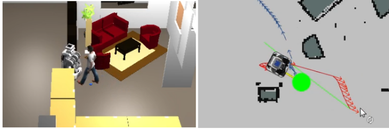
Figure 2.5: Narrow passage scenario in which the robot backs off to make way for the person [53].
