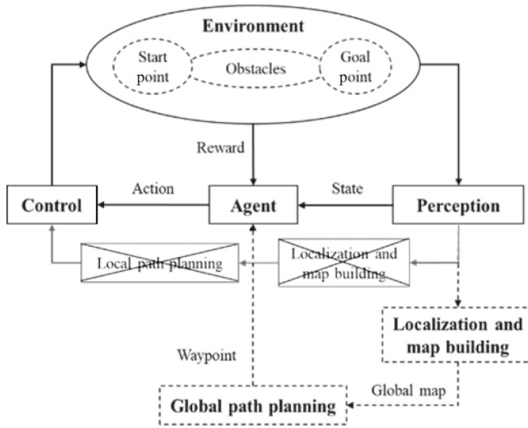
Figure 2.2: DRL-based navigation framework[68].
