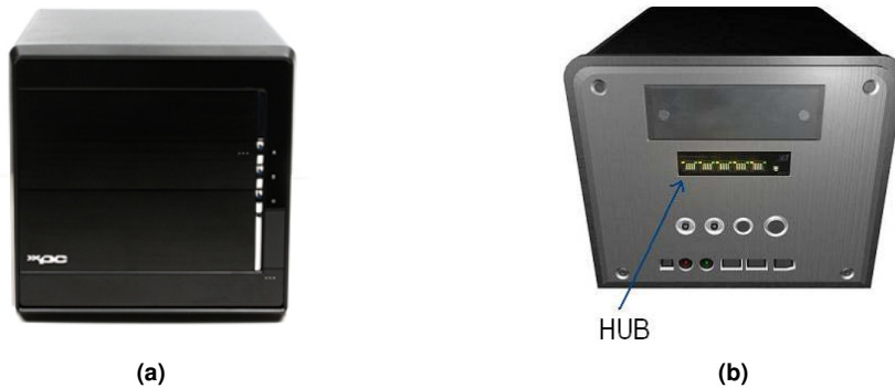
Figura 2.2: Computer/server (a) e l'HUB integrato (b)
