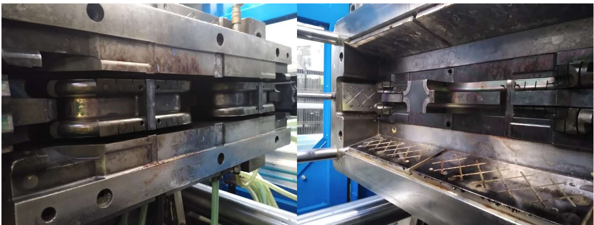
Fig. 31: Bridge corner's mold
